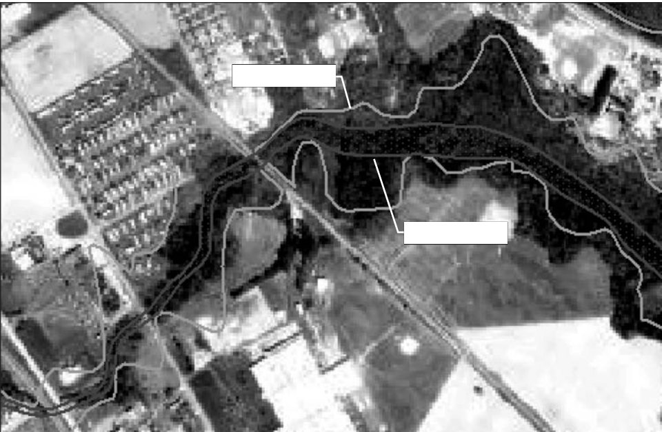
Figure C-6. Floodwaters in the floodway (dark gray) will have higher velocities than those in the flood fringes (between black and gray).
