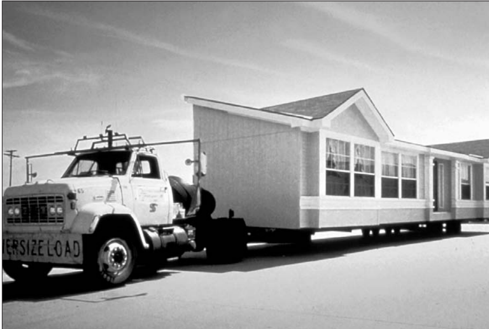
Figure 2-4. One section of a double-section manufactured home being transported.
